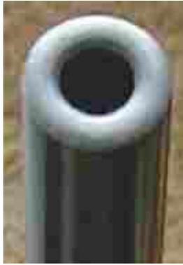
**The original factory crown just before cutting it to an 11 degree target crown.**
