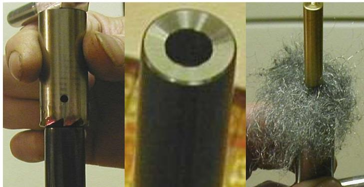
**Left - finish cutting is performed with increasingly lighter pressure as cutting progresses until almost only the weight of tool is applied to the muzzle.**
