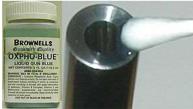
**Left - after using alcohol to degrease the muzzle OXPHO-BLUE from Brownells is used to cold blue the muzzle.**
