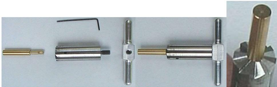
**Left - .308 caliber brass pilot, 79 degree muzzle crowning cutter, cutter handle and allen wrench for tightening pilot to cutter.**
