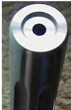
**Picture shows a 'step' type target crown on a Green Mountain .22 calibre barrel.**
