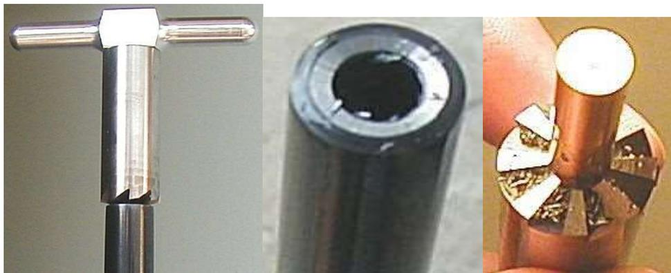
**Left - crowning cutter with pilot inside bore, ready to start cutting.**
