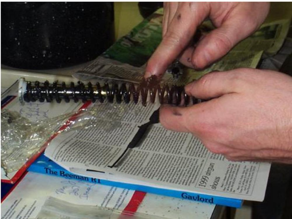
Slide the spring into the receiver and into the piston. That's a nice, safe place to keep it while you clean your hands and get your spring compressor ready. Compress in the spring and
