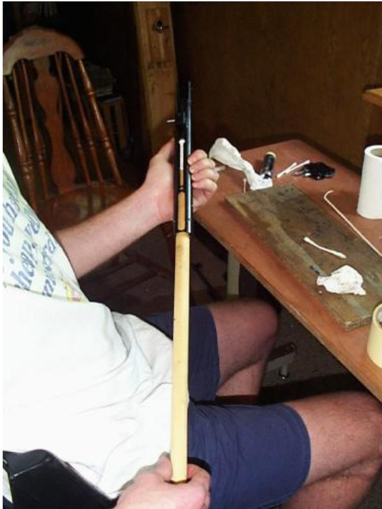
After you've got the gun all clean, it's time to lube up the new parts. Moly the sides of the piston seal and piston. Don't put it on too thick, but do put on enough to allow for losing some against the receiver wall as you slide the piston home. Be careful to avoid cutting the seal on any openings in the receiver tube. Save tarring the spring for a minute.
