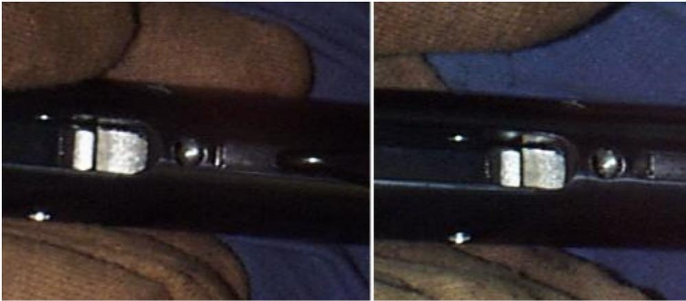
The picture on the left is the engagement you can get with the Weihrauch spring; the picture on the right is Maccari's. It's not clear in this picture, but on the right, with the factory spring, almost the entire cut of the notch has emerged--just a hair of it remains concealed. About 1/16" inch or slightly less of the notch is concealed when using Maccari's spring and guide. If this is the case for you, I will provide a solution at the end of this account.
