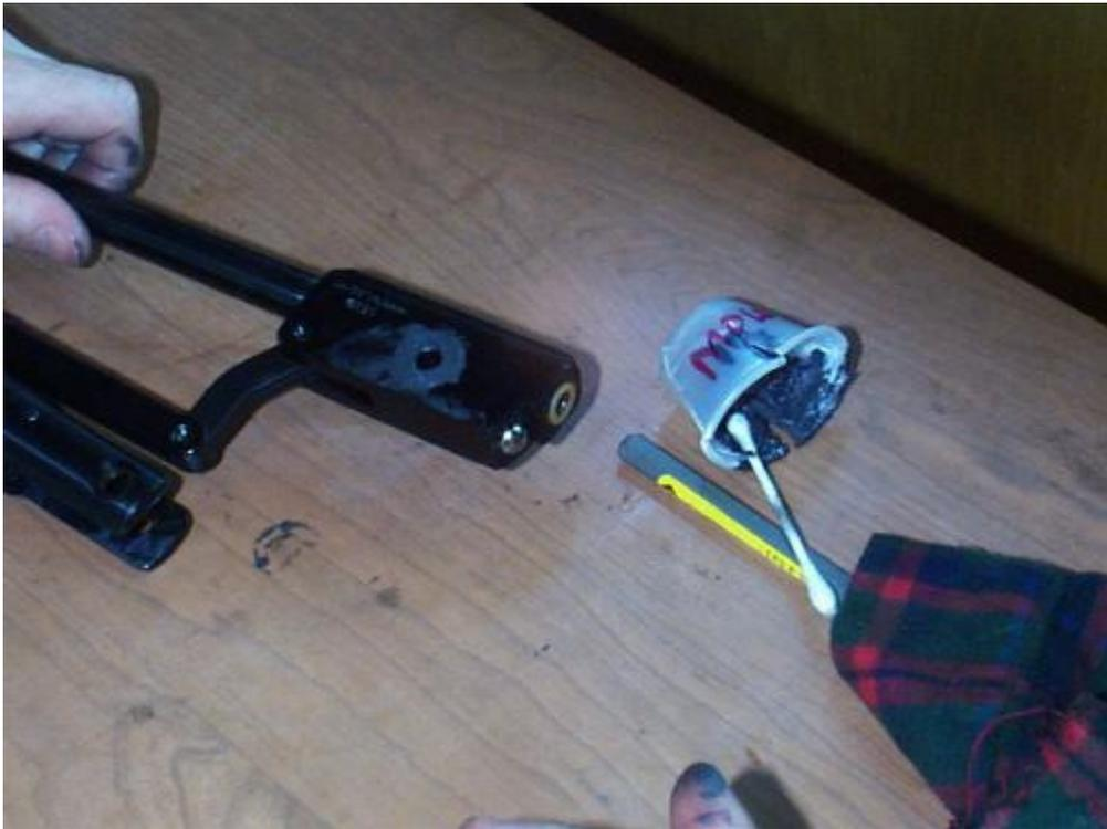
Using your punch or something pointy and sharp, pull the disks into proper alignment. Insert the bolt, remembering that it goes in from the left, and it's nut and locking attaches from the right. Just snug it down to prevent fall-apart.
