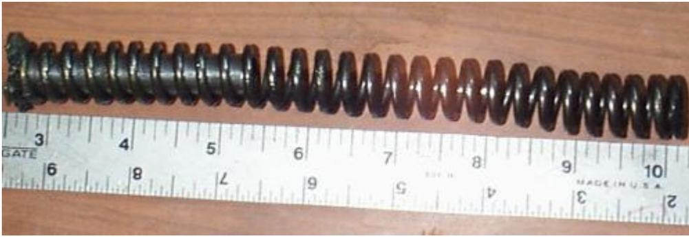
As you can see in the next photo, Maccari's spring is slightly longer than the Weihrauch spring, and it's got a thicker flange on the spring guide. The Weihrauch spring guide is more loosely fitting.
