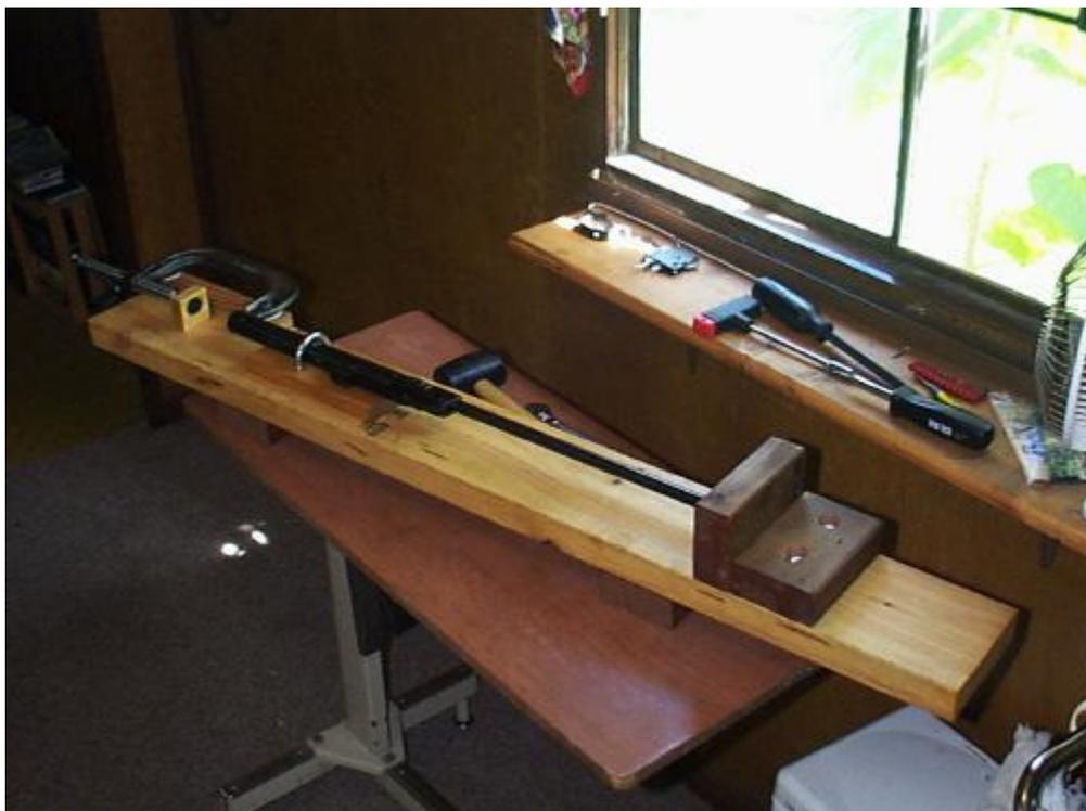
To remove the spring, apply pressure with the spring compressor to the endcap then unscrew the single screw that holds the endcap into the gun.
