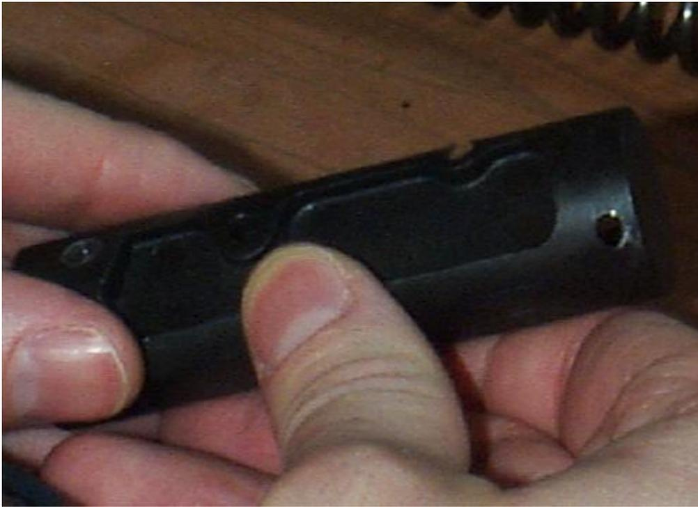
Remove the action from your compressor. Next you'll need to remove the cocking link so that you can free the piston. Begin by driving out the little bridge pin that retains the cocking arm--use the 1/8" punch and rubber mallet again here.
