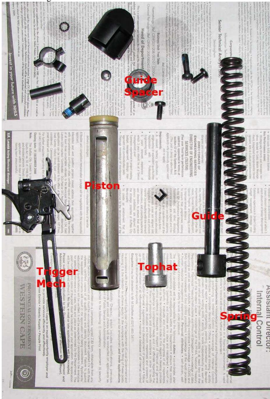
What your aim is with the parts is to make them fit each other and to de-bur all the stamped metal parts. This includes the inside of the piston and the receiver (the main part
