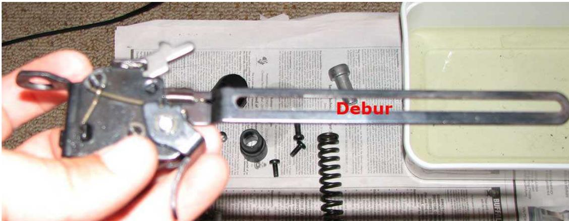
Remove the beartrap by taking off the circlip and unhooking the spring. Take note how it is attached.
