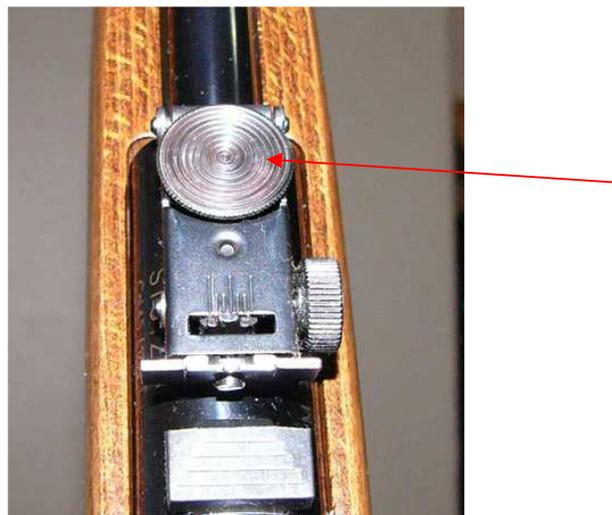
The sight will then be able to flip forward revealing a small bolt attaching it to the barrel. Unscrew and lift it off. Put it in a safe place.
