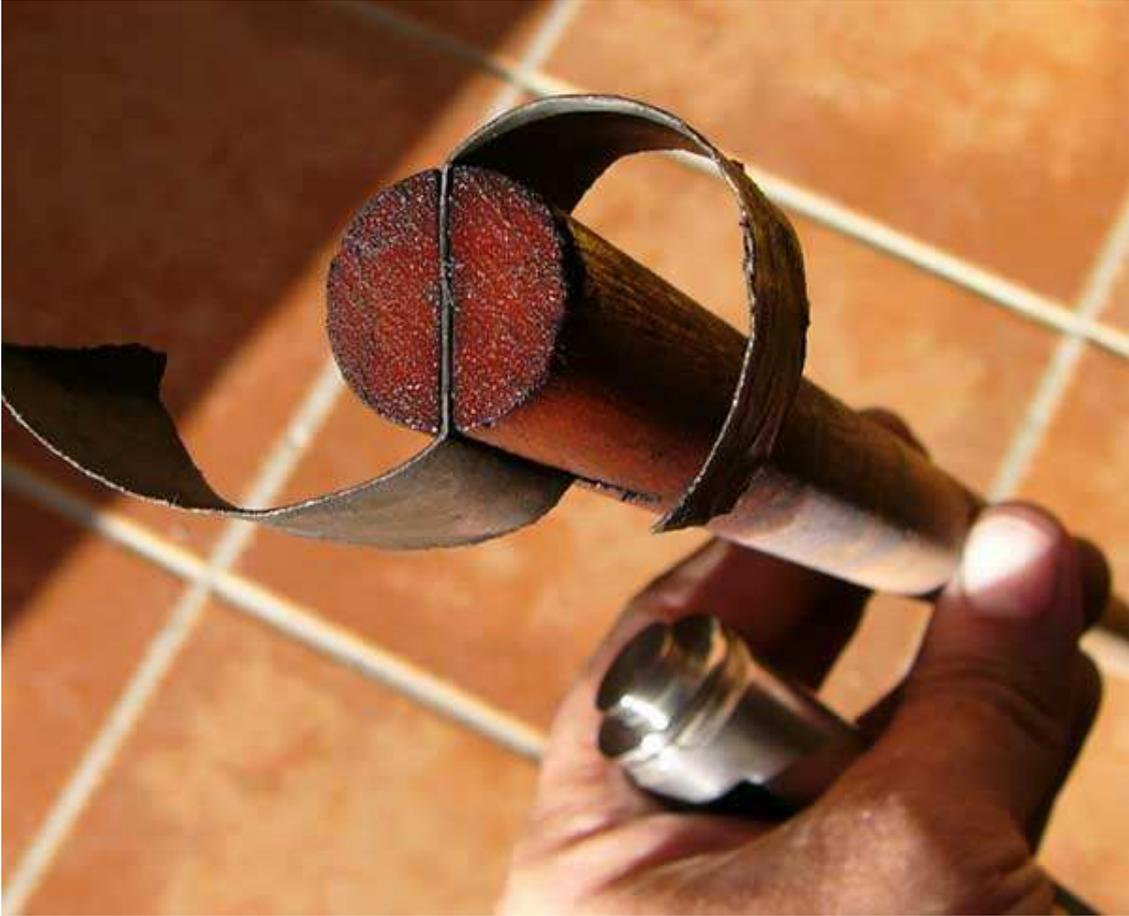
Now sand the inside of the piston using a rotating motion
