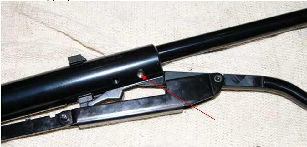
9. Remove the barrel/lever from the action. You will find on the bottom of the receiver a groove for the cocking arm to operate in. In the front it will have a round hole. Remove the cocking arm by sliding the foot to this hole and pulling it out.
