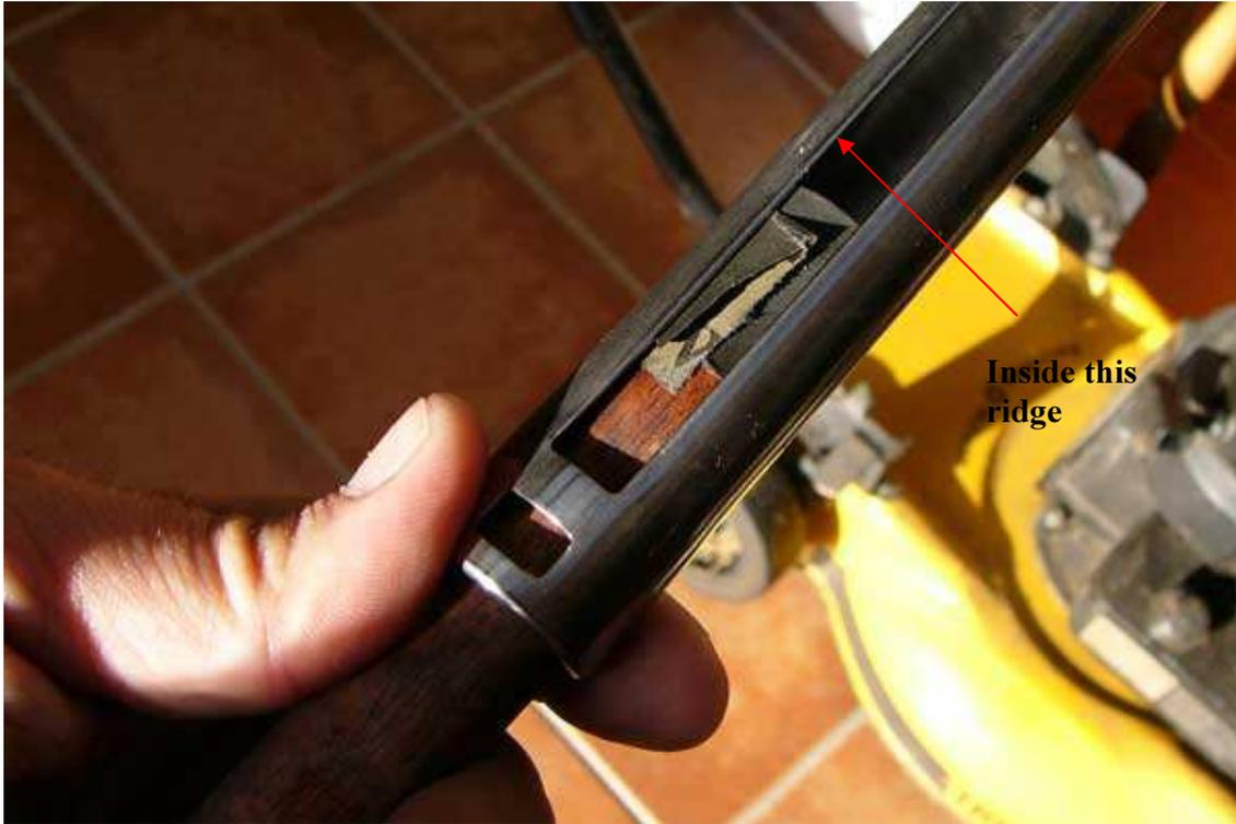
If you have a polishing wheel you can now polish the outer surface of the piston. You should also polish the lip where the trigger catches to ensure a clean break
