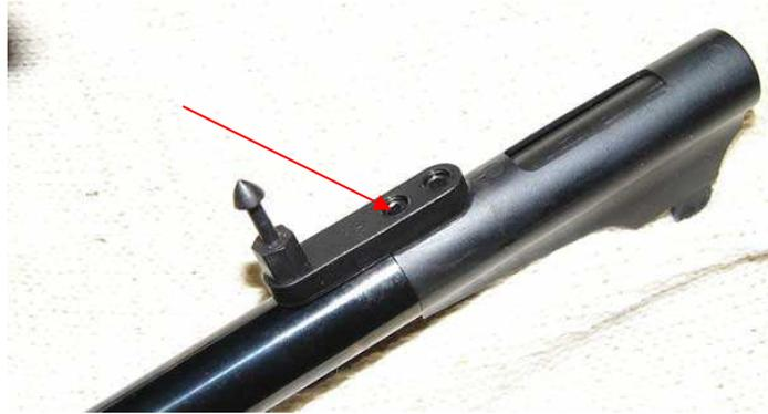
7. Remove the end cap at the rear of the receiver. It is held in place by the trigger assembly screw. The big round thing that looks like a nut with two flat sides behind the trigger assembly. Undo this screw and remove the end cap.
