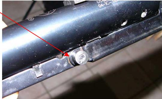
6. Place the stock somewhere safe! Again, it will be sad to scratch it. Now remove the sights – if your rifle has any. You do not want these to break while you are working on the rifle. On the rear sight of the Stutzen, just unscrew the elevation adjuster. Here still pictured before taken from the stock.
