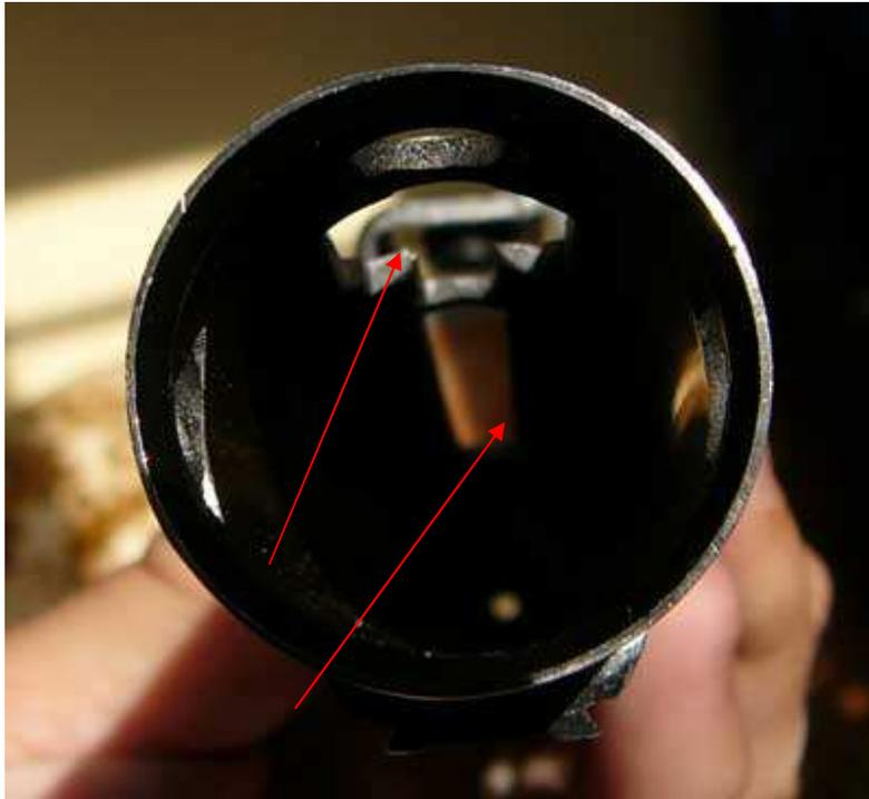
You can then use you dowl sander creation to clean up the inside of the receiver where you just de-burred. Clean the receiver very well using your dowl creation and alcohol, as anything left behind will be pushed into the piston chamber when re-assembling.
