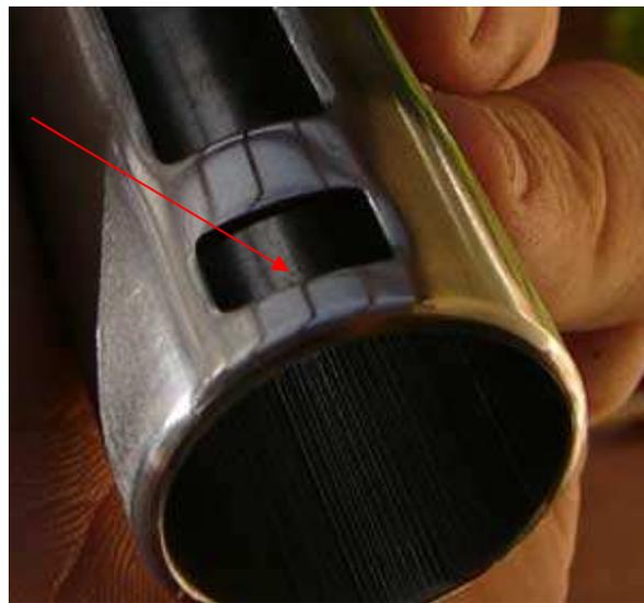
Why are we polishing these surfaces? To reduce rotational force. We are trying to prevent the spring when uncoiling from trying to rotate the gun and rather just rotate on the polished surfaces.
