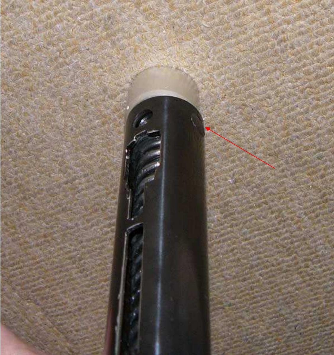
12. You can remove the guide, spring, tophat and piston now. Everything but the piston will just "fall out the back" so to speak. The piston you can push backwards gently with a screw driver in the cocking slot. Be gentle so that you do not scratch anything.
