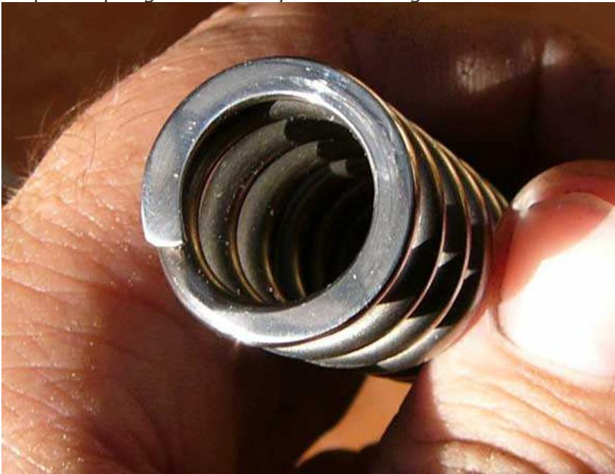
4. Move on to the Rear spring guide. Sand the outside surface to mirror finish and de-bur the tip of the guide. And clean it out with alcohol.
