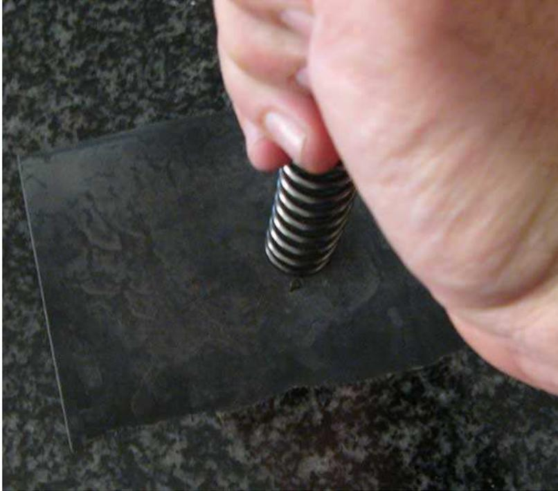
Go to 1600 and you will find the surface starting to resemble mirror finish. This will help the spring rotate freely when coiling.
