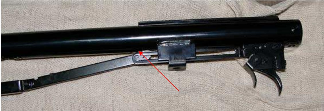
10. Now turn it 90 degrees with the sliding arm and you will be able to remove it. On the stutzen, due to the way the mounting bolt mounts the stock to the receiver, I have to remove the trigger assembly 1<sup>st</sup>. To remove the trigger assembly slide it rearwards in the receiver and pull it out through the recess at the rear bottom of the receiver.(right in front of where you unscrewed the trigger assembly screw.
