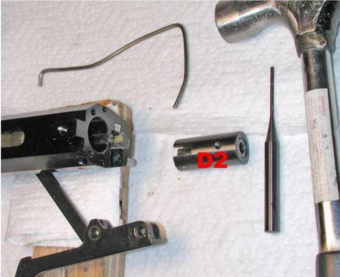
Access to the hinge pin is limited. A slim straight and a curved punch is needed. Carefully Tap the pin out from the bottom just enough to remove the cocking lever.
