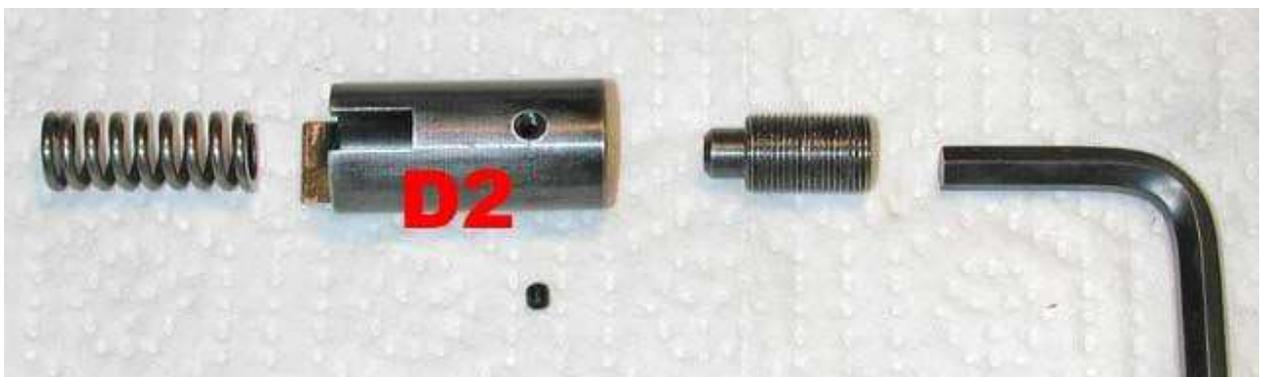
Clean off the Loctite on the adjustment screw. If you are keen, polish off the sharp edges of the shuttle and smooth out the hammer spring ends.
