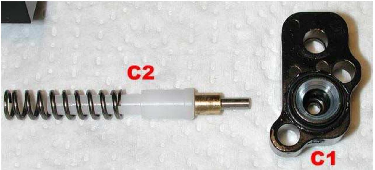
Part C1 is the part that directs the compress air to the pellet. It contains the breech, probe seal, porting and valve seat. Two hex bolt hold this part to the front action block C.
