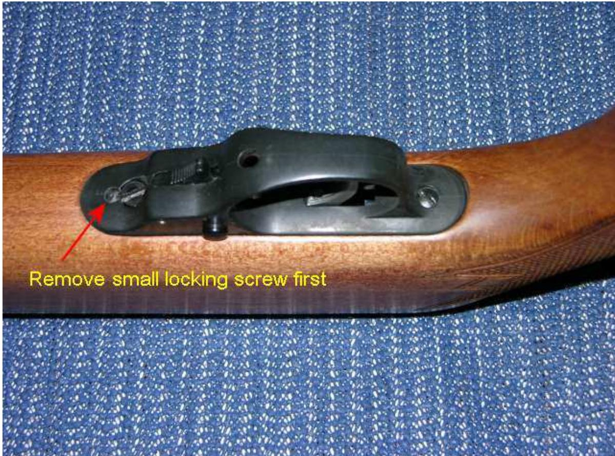
Before removing the bigger screw it would be a good idea to put a mark on the screw head and trigger guard, so that when you put it back you know exactly how far to turn it to get it back to the same position.
