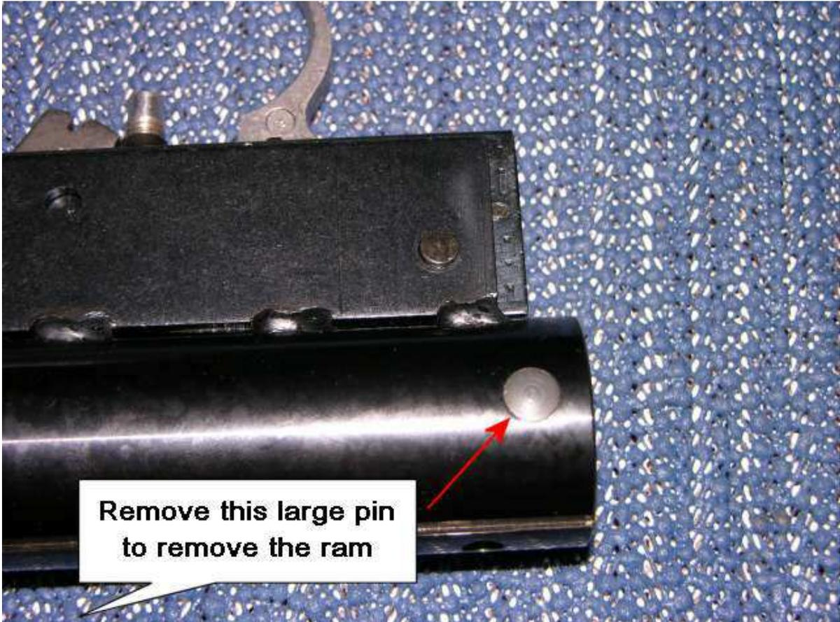
**When you have the large pin out, push the piston/ram out of the cylinder via the cocking slot under the cylinder.
