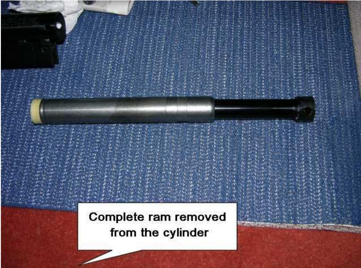
**The ram can now be pulled into two pieces to expose the inner part of the piston.**
