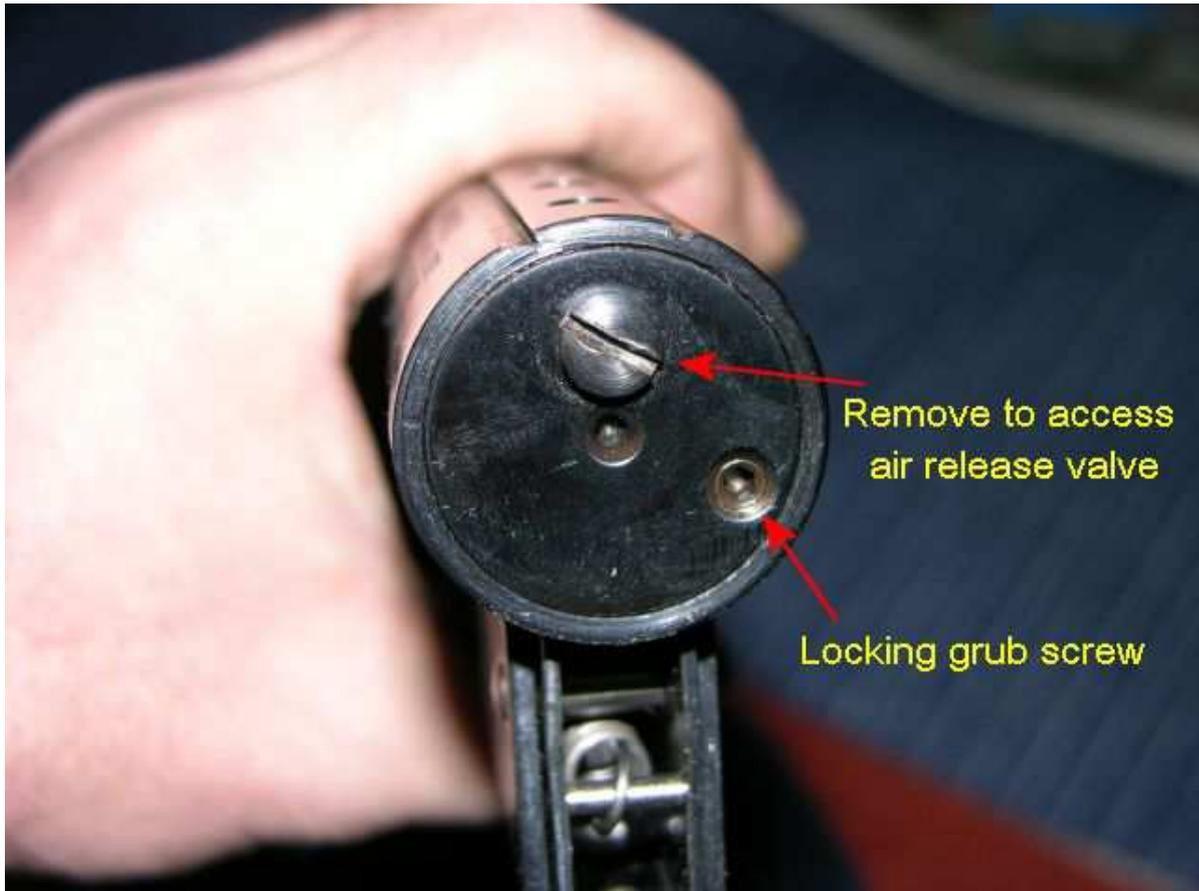
**Once you have the screw out of the way you can now start to let the air out from the ram by tapping gently on flat bottomed object positioned on the valve pin.
