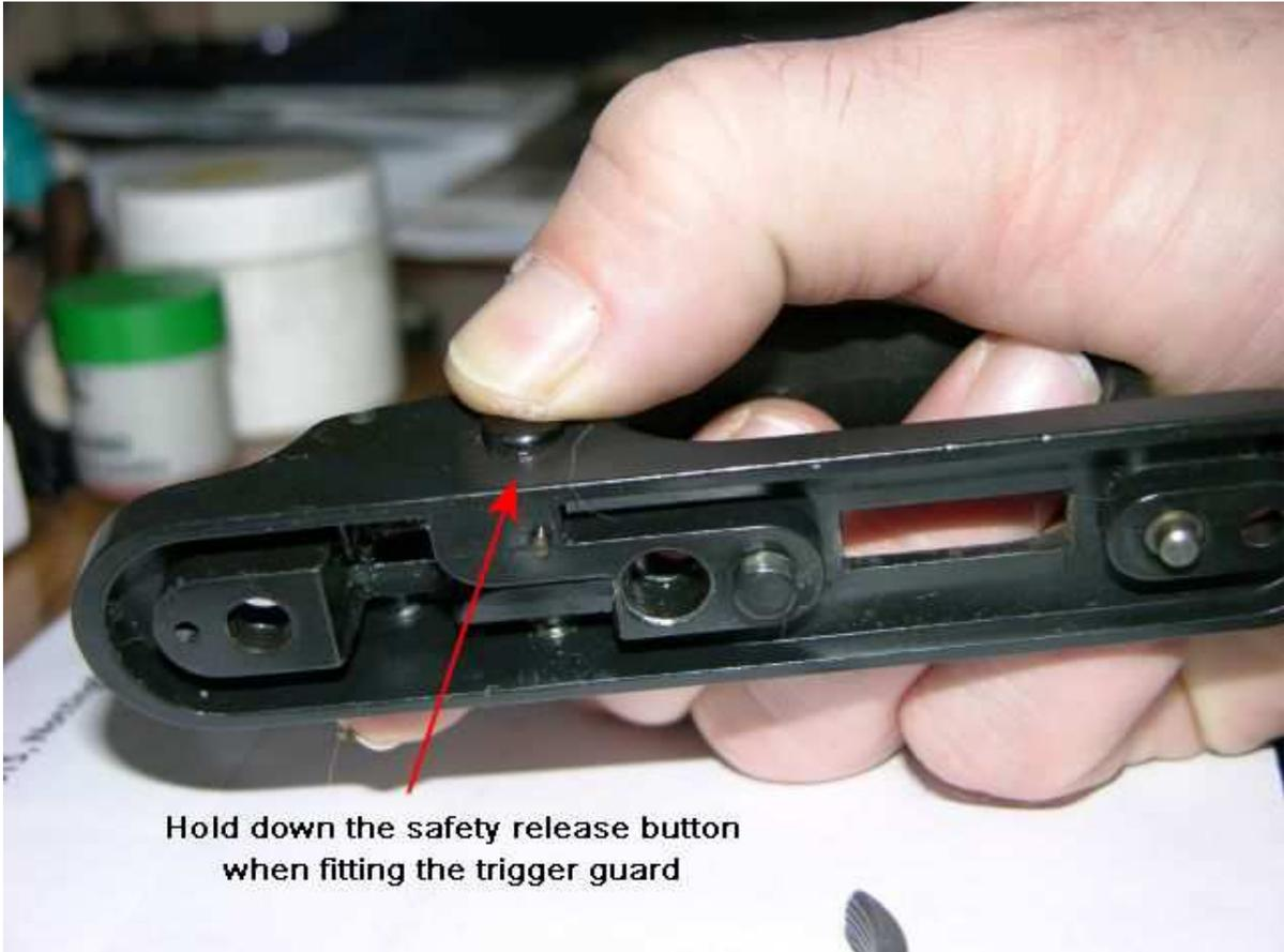
**If your trigger guard feels like it won't go back on you may need to pull the trigger blade about 1 or 2mm just enough so that it clears itself away from the gap in the trigger guard housing.**
