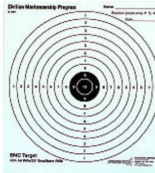
*The BMC target is printed on a 6 1/2”x7” card, has a 15.25mm 10-ring and nine additional scoring rings that are each 15.25 mm larger.*
