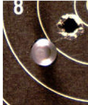
*When a scoring gauge is inserted in a shot hole, it is possible to see exactly where the edge of the shot hole lies.*
