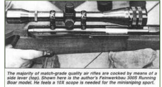
The majority of match-grade quality air rifles are cocked by means of a side lever (top). Shown here is the author's Feinwerkbau 300S Running Boar model. He feels a 10X scope is needed for the minisniping sport.
