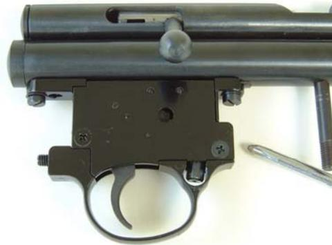
3. Use a #2 Phillips-head screwdriver to remove the two **Casing Plate Screws**. Lift off the **Casing Plate** to expose the trigger mechanism.
