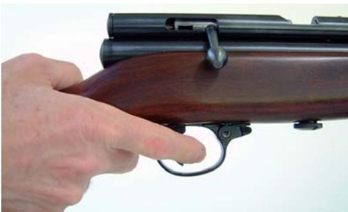
9. *Point the rifle in a safe direction* and pull the trigger. A mild report 'pop' verifies the weapon is now charged with CO<sub>2</sub> and is ready for shooting.
