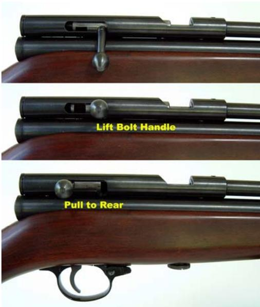
3. Open the **Bolt** as illustrated above. Opening the bolt leaves the loading chamber open to inspection. More importantly, *retracting the bolt prevents dangerous accidental piercing of the rearward-facing CO<sub>2</sub> cartridge*.
