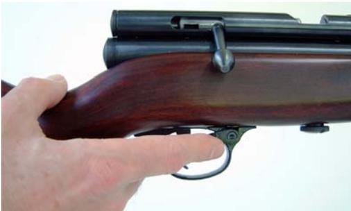
2. Apply the **Safety** by swinging it to the rear as shown above.
