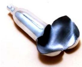
When the cartridge is nearly depleted, the transition point marks the end of useful life. This is the point at which all of the *liquid* CO<sub>2</sub> has been consumed.
