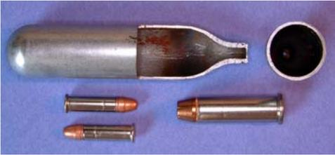
The Powerlet contains a considerable amount of energy (over 280 ft-lb or 380 Joule). This is approximately equivalent to two high-velocity .22 long-rifle shells, or one .38 Special (+P) cartridge. To place this in another perspective, the contained energy is sufficient to light a 100-Watt bulb for nearly four seconds. Any one of these equivalents is clearly capable of injuring you; the CO<sub>2</sub> cartridge must be treated with care and respect!
