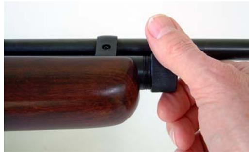
5. Screw the **Gas Tube Cap** back on fully; this will pierce the forward-facing CO<sub>2</sub> cylinder. When the cap has seated fully hand-tight, back it off a quarter-turn. This will allow the CO<sub>2</sub> to flood the **Gas Tube**. *Do not forget to back off or the forward-facing cartridge will remain sealed by the **Gas Tube Cap**.*
