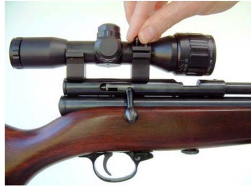
3. Fit the scope into the bases. Slide one of the bases until the spacing is 'right' about the scope's central *turret*. Add the ring caps, but only hand-tighten their screws.
