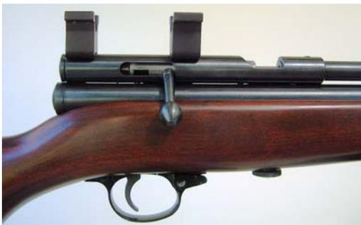
2. Mount the bases to the receiver. Only hand-tighten the clamp screws; you need the bases to slide freely at this point.
