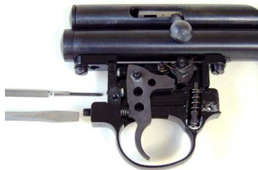
4. Use a 2 mm flat jeweler's screwdriver to adjust the **Sear Engagement** and **Overtravel** screws. Use a 3/16” flat screwdriver to adjust the **Tension** screw.
