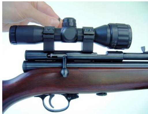
4. Hold the rifle in firing posture. Slide the scope back and forth until you achieve a position that lets you see through the optic with the least "tunnel vision". Lock the base screws at this location. Twist the scope body to align the graticule vertical line up and down. Then tighten the cap screws.
