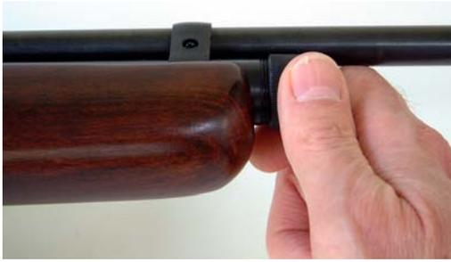
1. Verify that the **Gas Tube Cap** can be loosened *by hand*, as shown above. *Never* use a tool to rotate this cap. A tight cap indicates dangerously high gas pressure remains within the **Gas Tube**.
