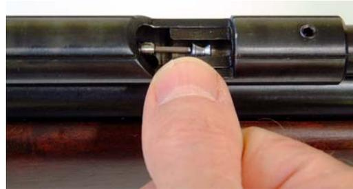
2. Insert a **pellet** of the proper caliber into the open breech. Make certain the pellet enters *nose-first with the fan-tail skirt to the rear*, as shown.
