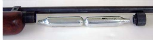
4. Unscrew the **Gas Tube Cap** from the **Gas Tube** and set it aside. Slide two **12-gram CO<sub>2</sub> cartridges** into the **Gas Tube** back-to-back as shown above. Note, for shorter shooting sessions, load an *empty* cartridge as the rearward-facing (first installed) cartridge. This will give approximately 30 full-power shots.
