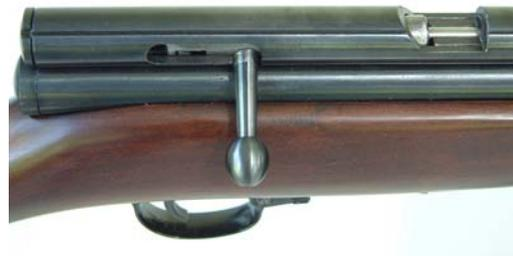
3. Push the **Bolt Handle** fully forward and rotate it down. This seats the pellet into the rifling and seals the breech. The weapon is ready to fire.
