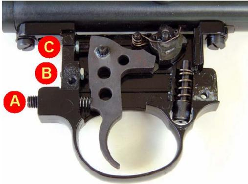
The QB78 trigger features three adjustments:
