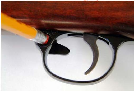
1. Place the **Safety** lever in the SAFE position and push it out of the **Trigger Casing** from left-to-right. Use the eraser-end of a wooden pencil as the dismounting tool.
