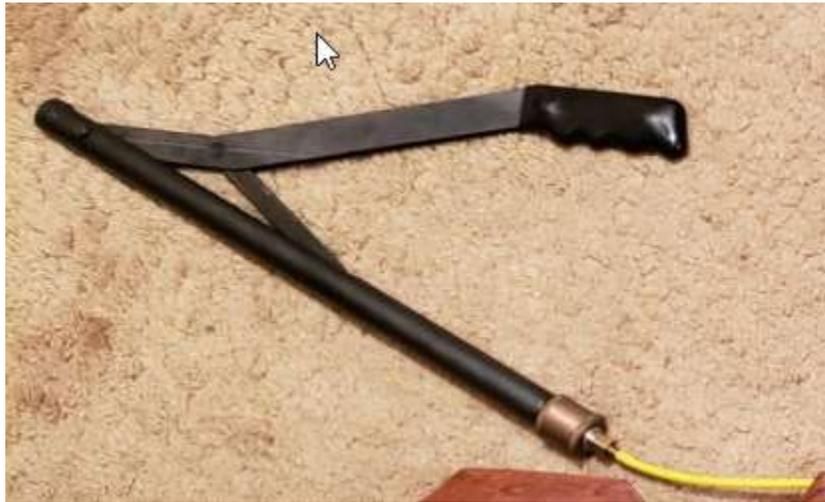
6. Try firing gun over chrony. If the chrony registers, try another 10-15 pumps until you reach the desired velocity. For a .22 with a 21 grain pellet, 775fps equates to 28fpe. Expect to pump 80-100 times to reach your desired velocity.
