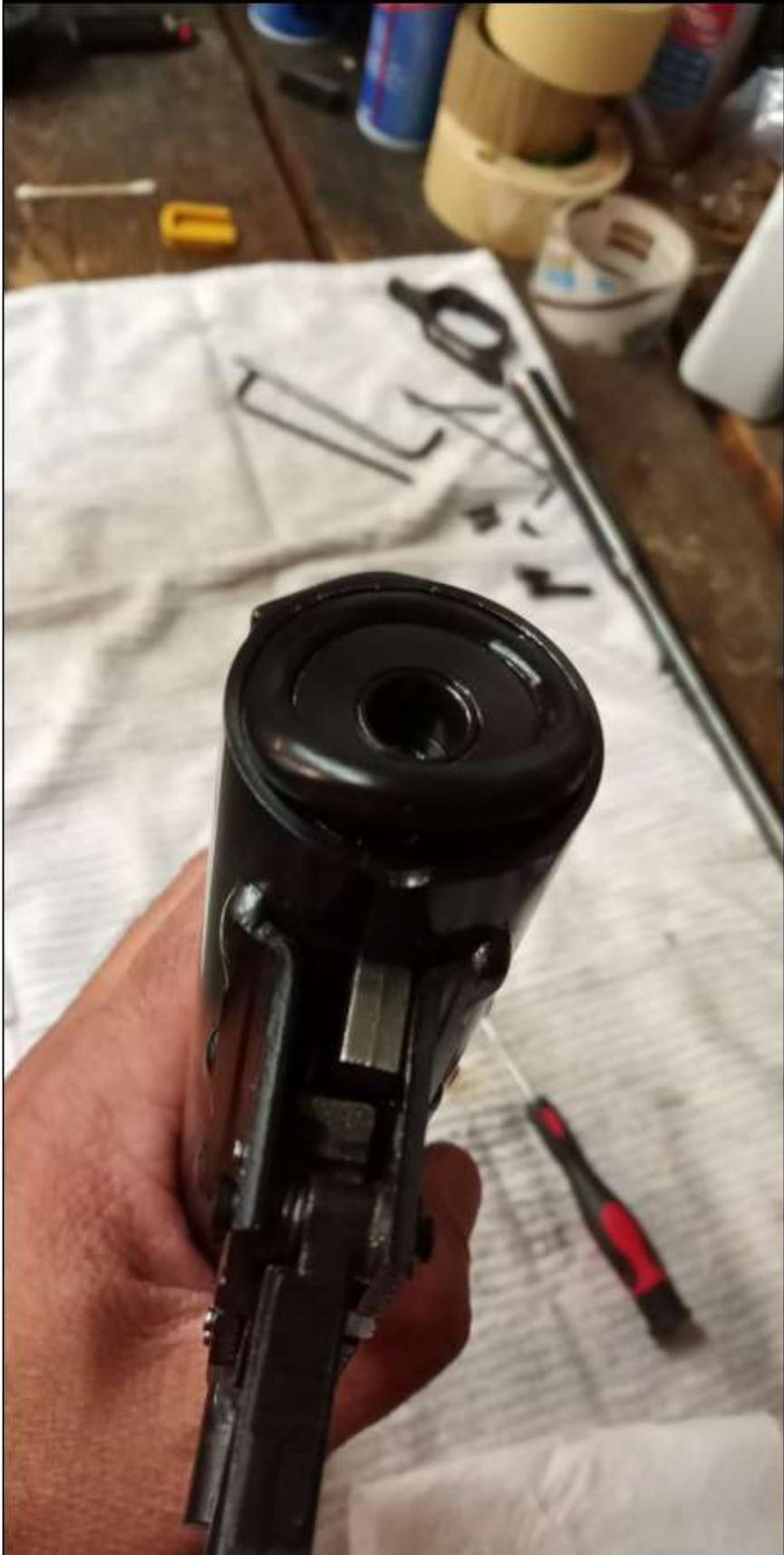
8. Remove snap ring holding the ram in place. Depress ram so you can grip the snap ring with the snap ring pliers. Earlier versions had a cross pin to retain the ram.
