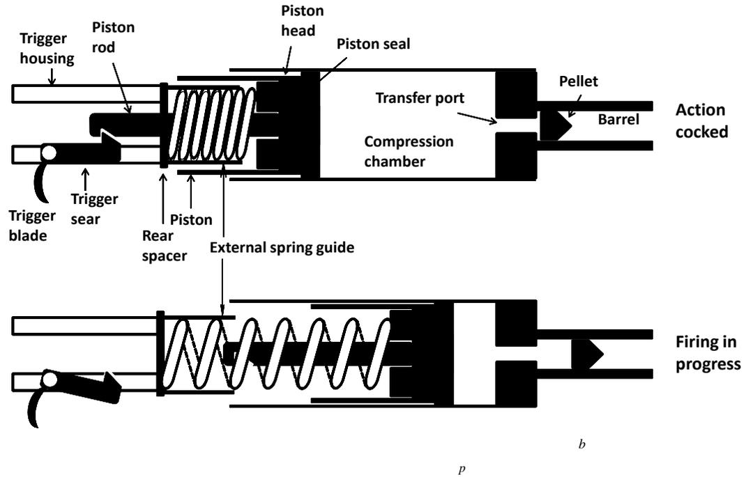
A difference between the action shown in Figure 2 and the same action discussed in Ref. 1 is the presence of a spring guide. Spring guides can be external, internal, or a combination of both. The spring guide in Figure 2 is external and consists of a tube within which the spring coils slide as the spring expands and contracts. An internal guide would be similar, only it would be inside the spring, and the cocking rod (piston rod) would slide inside the guide<sup>1</sup>.
