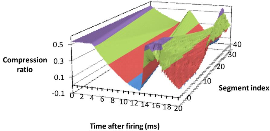
The flat, triangular area starting at time zero in Figure 6 represents the finite element segments not yet reached by the expansion wave originating at the front end of the spring (index  $40^1$ ). From the plot, you can see that the wave front takes between three and four milliseconds to reach the rear of the spring. This is in keeping with the theoretical value of 32.23 m/s
