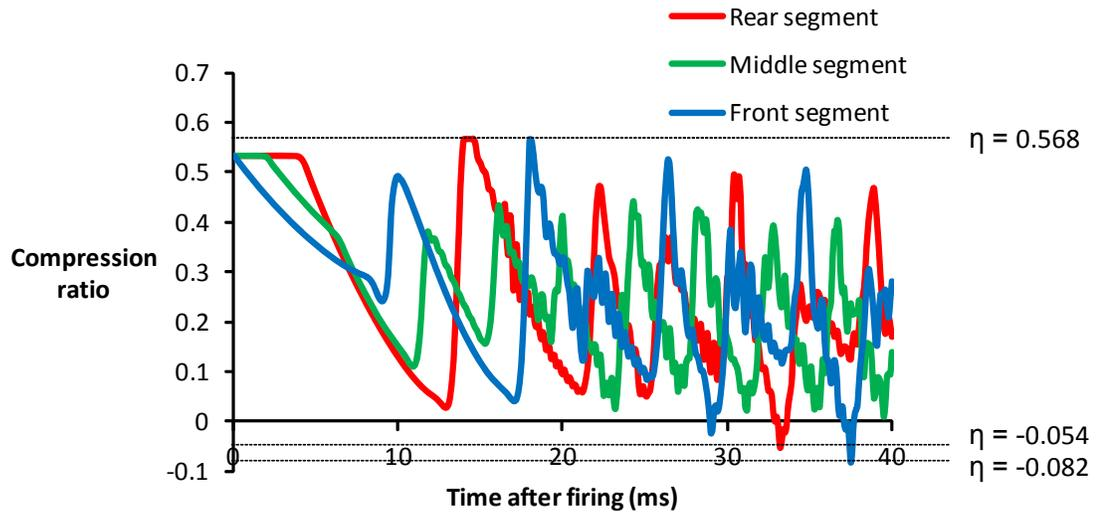
Notice that in some instances the spring segments are, during brief periods, in tension (negative compression ratio). This surprising result adds to the range of dynamic stresses that contribute to fatigue<sup>1</sup>. The red line in Figure 8 clearly shows that the rear segment compression ratio tops off at 0.568 when the coils clash.
