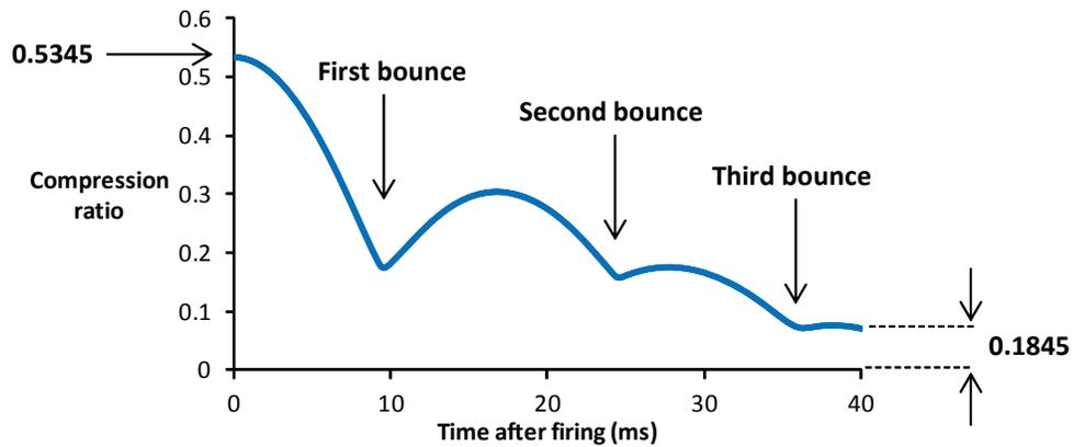
Even in the absence of friction between spring and guide, the spring will eventually settle down in the un-cocked configuration as energy is dissipated by friction between the piston and the chamber walls, as well as by heat formation due to air flowing non-isentropically in and out of the chamber through the breech.
