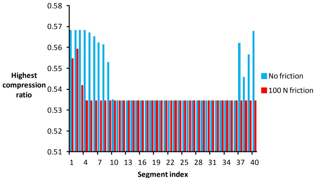
It is clear from Figure 12 that the effect of friction is to make the highest compression ratio fairly uniform across all spring segments. Intuitively, we expect that the parts of the spring subjected to friction from the guide will see their compression swings ameliorated. What Figure 12 shows is that *all segments*, including the ones that are never in contact with the
