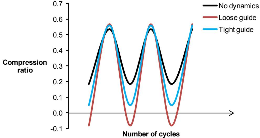
If the buzzing sound we hear when firing a gun with loose guides stems from the spring longitudinal vibrations, shown in Figure 8, then Figure 11 tells us that the use of a tight internal guide suppresses the buzzing sound by dampening oscillations that occur mostly *after* the projectile has left the barrel. This means the buzzing sound may be annoying, but it is not detrimental to accuracy.
